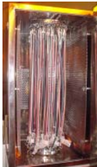
Fig. 2.2.2-2 Fabrication situation of the simultaneous aging specimens (Installation situation in the oven)
