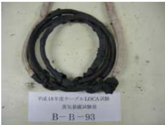
Fig. 2.4.2-22 Specimen B-B-93 after steam exposure test
