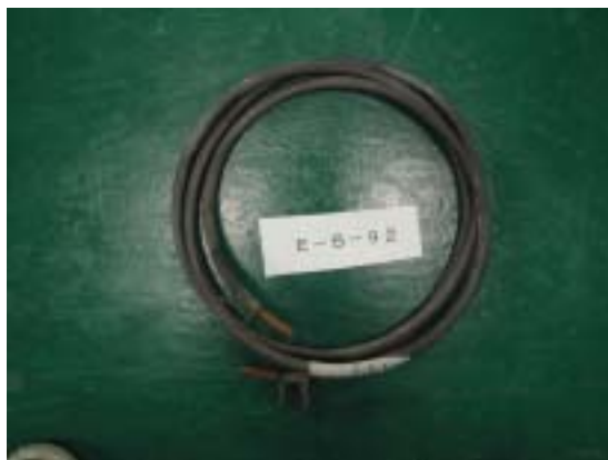
Fig.2.4.2-10 Specimen E-B-92 after steam exposure test
