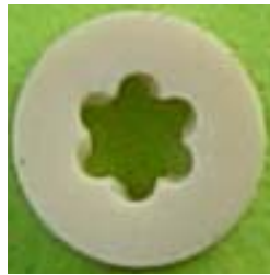
Fig. 3.1-7 Degradation situations inside insulator at the thermal aging (100°C) of PVC insulator (color change)
