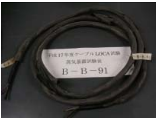
Fig. 2.4.2-4 Specimen B-B-91 after steam exposure test
