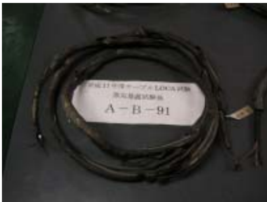
Fig. 2.4.2-2 Specimen A-B-91 after steam exposure test
