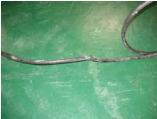
Fig. 2.4.2-14 Specimen H-B-91 after steam exposure test (at the bending work)
