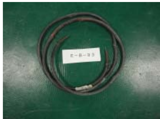
Fig. 2.4.2-11 Specimen E-B-93 after steam exposure test
