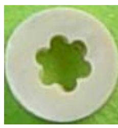
Fig. 3.1-7 Degradation situations inside insulator at the thermal aging (100°C) of PVC insulator (color change)
