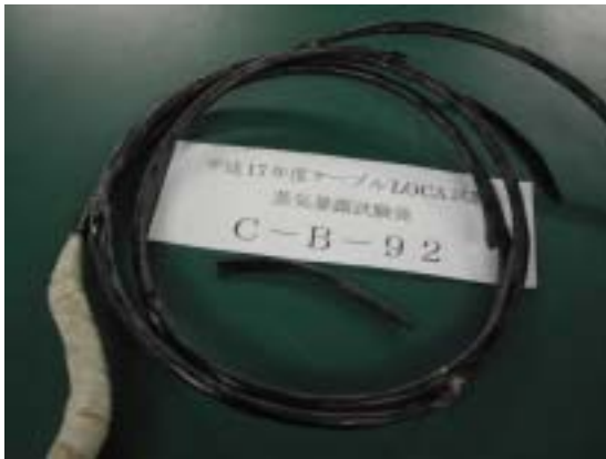
Fig. 2.4.2-6 Specimen C-B-92 after steam exposure test
