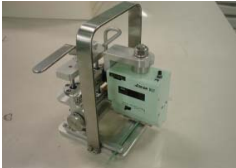
Fig. 2-5 Surface Hardness Meter for Cables Degradation Diagnosis
