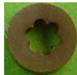
Fig. 3.1-6 Degradation situations inside insulator at the thermal aging (120°C) of SHPVC insulator (color change)
