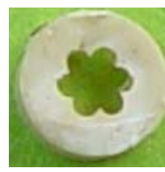
Fig. 3.1-7 Degradation situations inside insulator at the thermal aging (100°C) of PVC insulator (color change)
