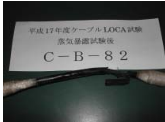
Fig. 2.4.2-7 Specimen C-B-82 after steam exposure test
