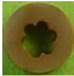
Fig. 3.1-6 Degradation situations inside insulator at the thermal aging (120°C) of SHPVC insulator (color change)
