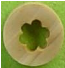
Fig. 3.1-6 Degradation situations inside insulator at the thermal aging (120°C) of SHPVC insulator (color change)
