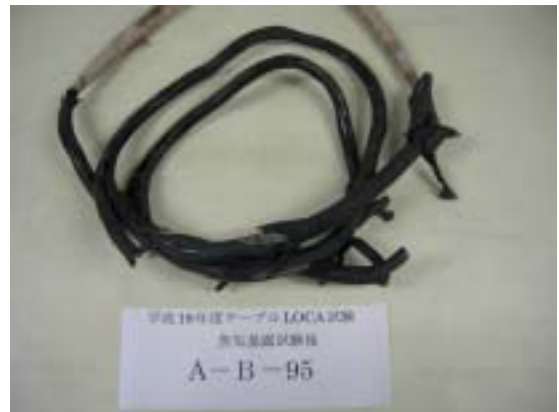
Fig. 2.4.2-21 Specimen A-B-95 after steam exposure test
