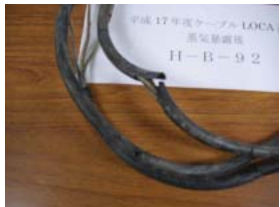
Fig. 2.4.2-15 Specimen H-B-92 after steam exposure test (after submerged withstand voltage test with bending of specimen)
